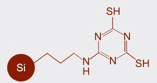
Loading: 0.83 mmol/g Surface Area: 525 m²/g Average Pore Size: 60Å Pore Volume: 0.79 cm³/g **Metals Targeted**
